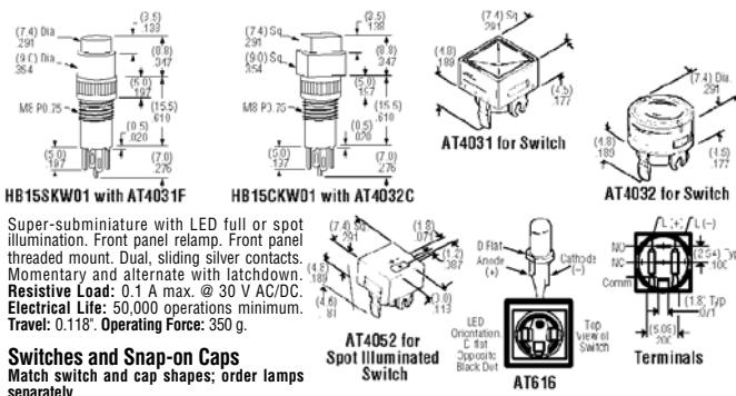
Super-subminiature with LED full or spot illumination. Front panel relamp. Front panel threaded mount. Dual, sliding silver contacts. Momentary and alternate with latchdown contacts. **Resistive Load:** 0.1 A max. @ 30 V AC/DC. **Electrical Life:** 50,000 operations minimum. **Travel:** 0.118". **Operating Force:** 350 g.
