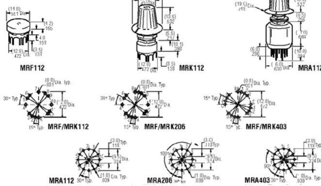
**MR Series Features:** Process sealed, all models break before make (non-shorting). **Rating:** MRF and MRK — 0.4 VA max. @ 28 V max. AC/DC; MRA — 250 mA @ 125 VAC. **Indexing:** 30°. **Electrical Life:** 10,000 detent operations min. **Operating Torque:** MRF and MRK — 50 g-250 g; MRA — 250 g-750 g. Supplied with black polycetal knob and with mounting hardware. **Bushing Diameter:** 6 mm (MRA and MRK).
