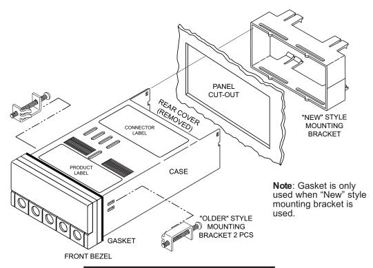
Figure 3-10. Meter - Exploded View
