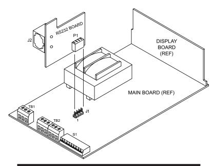
Figure 8-1. Installing the RS-232 Option Board
