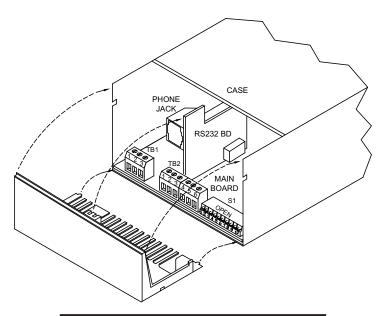
Figure 8-2. Protective Back Panel
