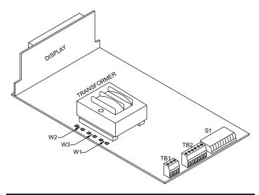
Figure 3-8. Main Board Jumpers (W1, W2, W3)
