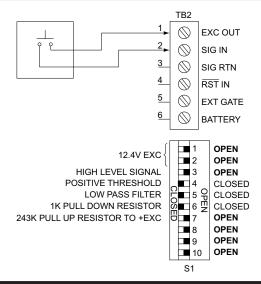
Figure 3-7. 2-Wire Contact Closure
