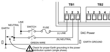
Figure 3-1. Electrical Connection for ac Power
