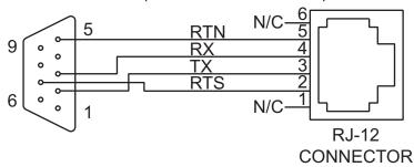
Figure 8-12. Meter Serial Port to a D-9 Connector
