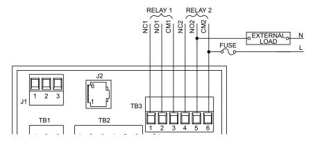
Figure 10-3. Electrical Wiring for Relay Connections
