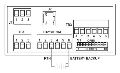
Figure 3-9. dc Power/Battery Backup
