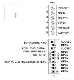
Figure 3-5. 2-Wire Magnetic Pickup (Low Level Signals)
