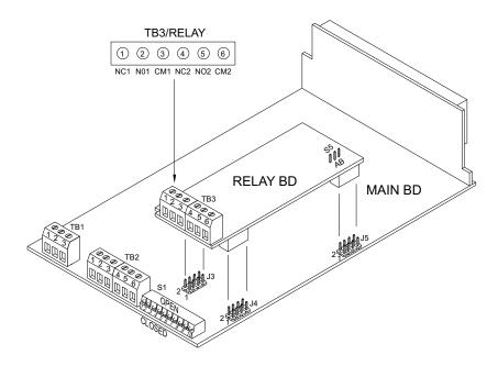
Figure 10-1. Dual-Relay Option Board
