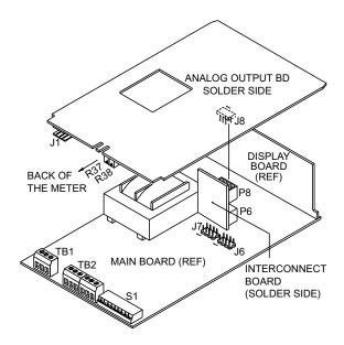
Figure 9-1. Installing the Analog Output Board
