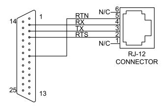
Figure 8-13. Meter Serial Port to a D-25 Connector
