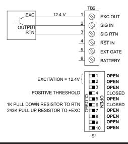
Figure 3-4. 3-Wire Sensor with PNP Open Collector Output
