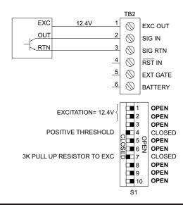
Figure 3-2. 3-Wire Sensor with NPN Open Collector Output
