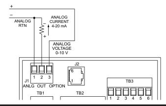
Figure 9-2. Electrical Wiring for Analog Output Connection
