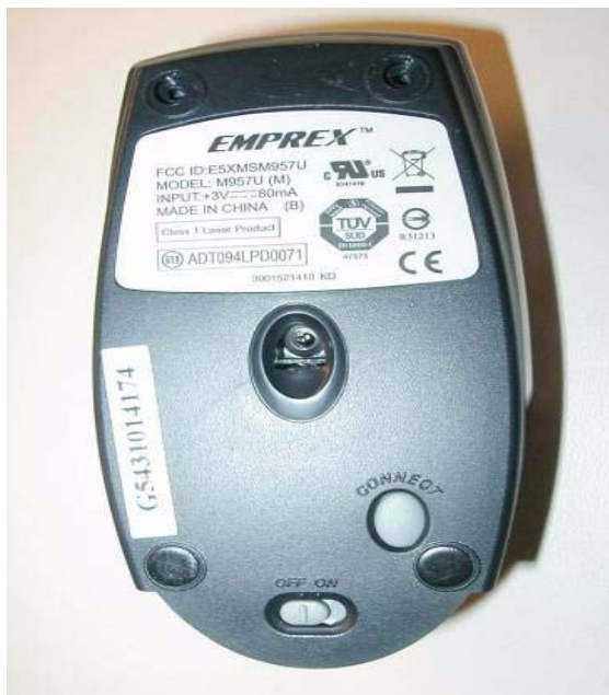
Figure 3-1. Bottom View Bind Button and On-Off Switch
