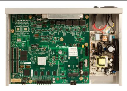
The P1025 RDB features 1 GB unbuffered DDR3 SDRAM, 16 MB NOR flash and 32 MB NAND flash, with the ability to boot from either NOR or NAND flash memory. The reference design board includes a built-in security accelerator and QUICC Engine for multiprotocol support. It also supports three Gigabit-capable ports via an SGMII PHY and two RGMII PHYs, two 10/100 Mb/s Ethernet ports, as well as two ports of USB 2.0, two 10-pin RJ45 RS485 ports and PMC connectors.
