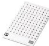
Marker cards, Card, white, labeled, Horizontal: Consecutive numbers 0 - 9, Mounting type: Adhesive, For terminal block width: 5.08 mm, Lettering field: 5.08 x 3.8 mm
