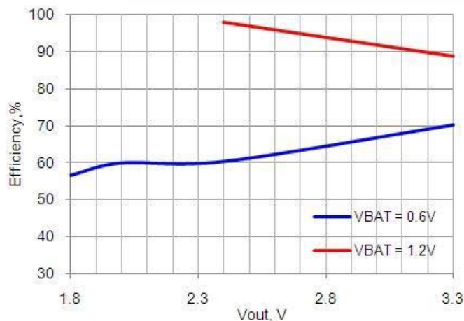
Figure 11-11. Efficiency vs V_{BAT}
