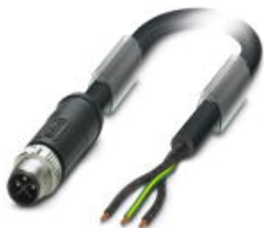
Power cable, 3-position, PVC, black, Plug straight M12 SPEEDCON, S-coded, on free cable end, cable length: 1 m, for AC current up to 16 A/230 V
