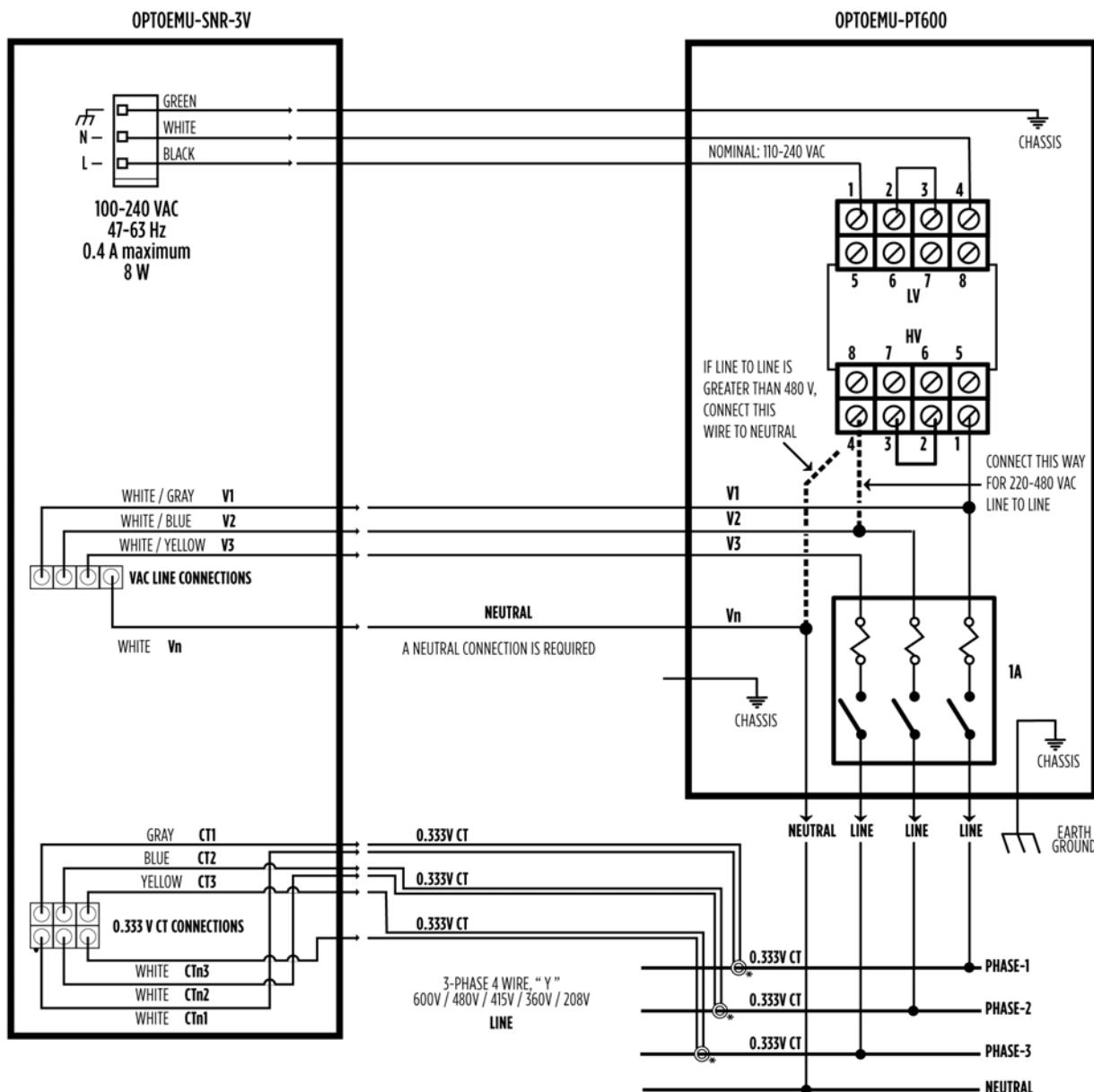
\*ARRANGE ALL OF THE 0.333 V CTS THE SAME WAY ON THE LOAD CABLES AND CONNECT THE CT SIGNAL WIRES IDENTICALLY (LABELED OR COLORED) TO THE WHITE WIRES.
