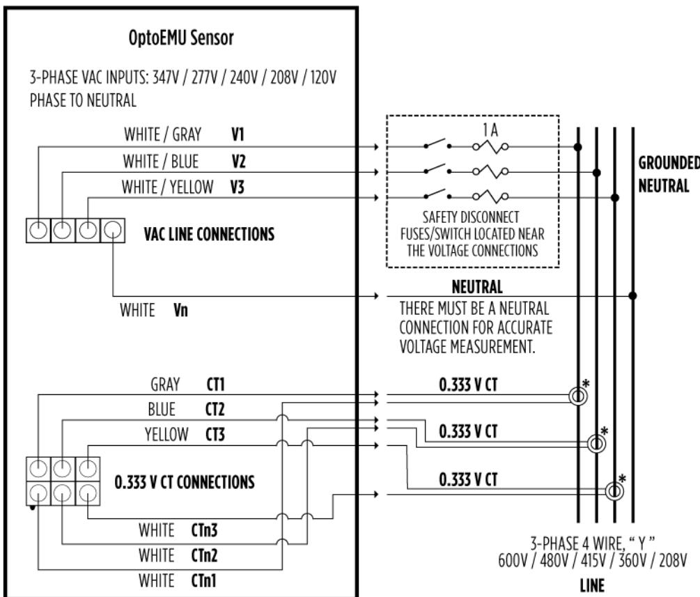
\*ARRANGE ALL OF THE 0.333 V CTs THE SAME WAY ON THE LOAD CABLES AND CONNECT THE CT SIGNAL WIRES IDENTICALLY (LABLED OR COLORED) TO THE WHITE WIRES.
