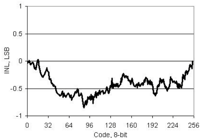
Figure 11-30. IDAC INL vs Input Code, Range = 255 \mu A, Source Mode
