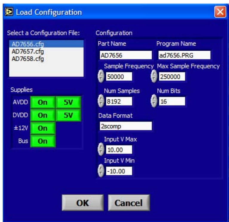
Figure 4. AD7656-1/AD7657-1/AD7658-1 Evaluation Software, Load Configuration Window
