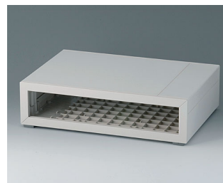
B2211017 MEDITEC D 160, without handle bar ABS (UL 94 HB) off-white RAL 9002 11.42"x7.87"x2.91" IP 40
