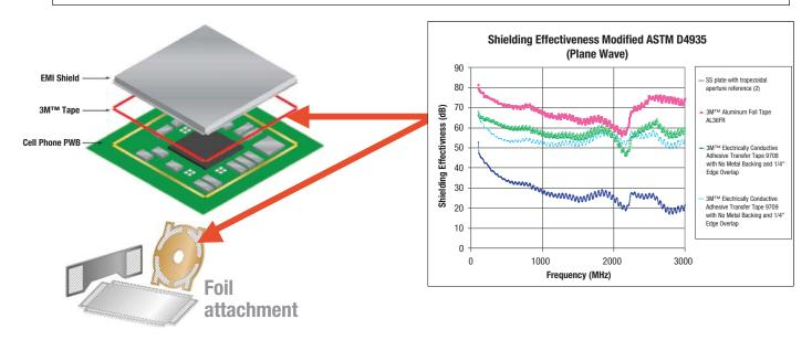
3M<sup>™</sup> Electrically Conductive Adhesive Transfer Tapes 9703, 9704, 9705, 9709, 9709S, 9709SL, 9712, 9713, 9723 and 7805 can provide FPC grounding and tapes 9707, 9709, 9709S, 9709SL and 7805 can increase the effective EMI Shielding through the bond line thickness leading to improved product EMI Shielding performance of the FPC.
