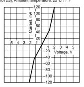
9. Off state leakage current
