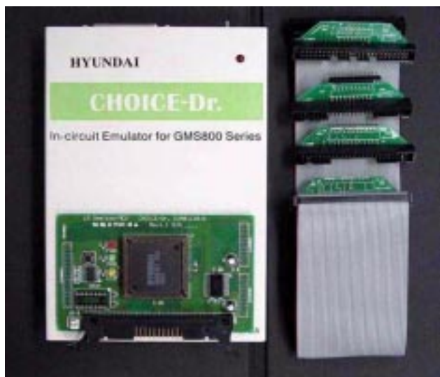
Figure 1-1 In Circuit Emulator CHOICE-Dr. TM
