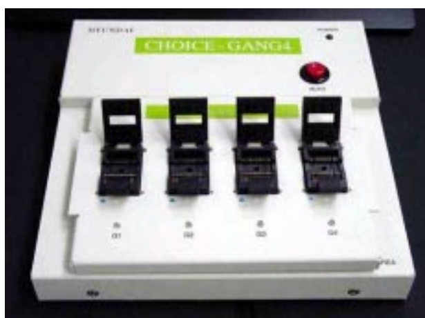
Figure 1-3 OTP Gang Programmer CHOICE-GANG4 TM
