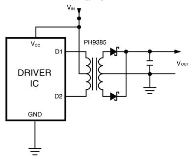
For a fixed 50% duty cycle mode of operation, the output voltage is simply determined by the input voltage and turns ratio. So, with the available turns ratios, a variety of output voltages can be selected. This range can be extended by implementing different topologies such as forward or bridge and can be used with controllers offered by different IC vendors for a number of different applications.
