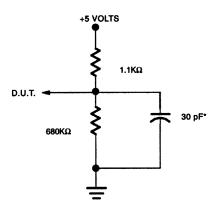
\* INCLUDING SCOPE AND JIG CAPACITANCE
