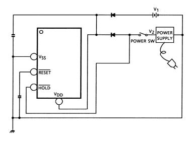
Note 11:  $V_1 = +3$  V: Battery supply
