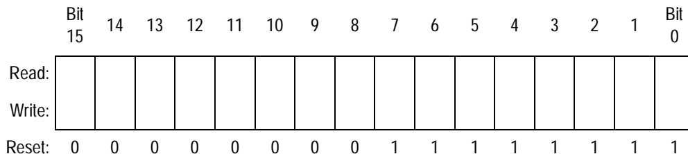
Figure 6-4. Stack Pointer (SP)
