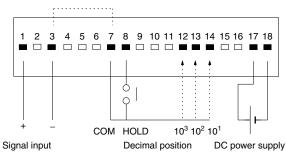
Note: 1. Terminals 3 and 7 of the AC and DC models are not internally insulated. Connect a relay with high contact reliability and insulation (with a minimum load current of 0.3 mA) or a photocoupler with high insulation (with a residual voltage of 1 V max. and a current leakage of 0.1 mA max.) to these terminals for external control.
