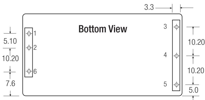
Pin Pitch Tolerance  $\pm 0.35$  mm
