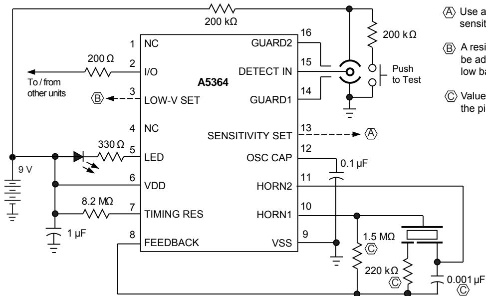
Ⓐ Use an external resistor to adjust sensitivity for a particular smoke chamber.
