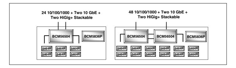
The BCM56504 is the fifth generation of the highly-integrated and cost-effective StrataSwitch and StrataXGS product line. The BCM56504 is a single-chip solution with 24-GbE ports and four 10-GbE/HiGig+ uplink ports.
