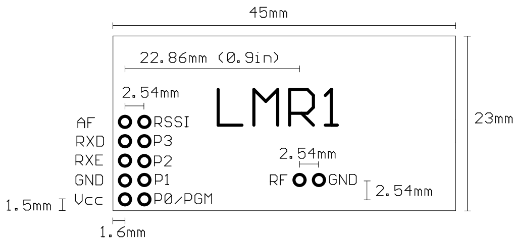
Figure 5: LMR1 footprint (top view)
