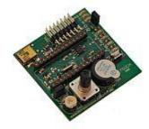
The Microstick Plus can also be used with PIC24F K-series Microsticks (DM240013-1, DM240013-2) except for the piezo buzzer, USB-UART converter, and CAN transceiver which are not compatible.
