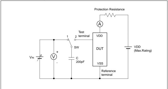
Note Charge voltage alternately switching 1 and 2 approximately 2 sec interval. This switching process is considered as one cycle.
