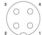
Pin assignment M12 socket, 4-pos., A-coded, view female side
