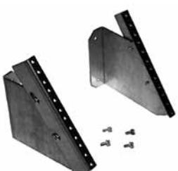
Swiveling rack angles drop 45 degrees to provide convenient access to equipment mounted on patch panels. Provide additional patch panel location in 36- and 48-in. (914- and 1219-mm) high cabinets. Made of self-grounding, plated 12 gauge steel. Mounting hardware included. Set of two.
