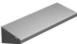
Shelves provide additional storage in 36- and 48-in. (914- and 1219-mm) tall cabinets. Made of self-grounding plated 16 gauge steel. 75 lb. (34.0 kg) load rating. RAL 7035 polyester powder coat finish.
