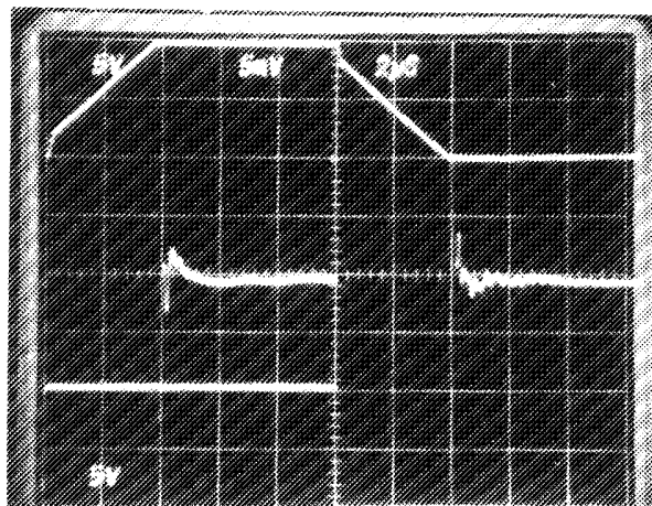
FIGURE 6. LARGE SIGNAL RESPONSE AND SETTLING TIME FOR CIRCUIT SHOWN IN FIGURE 23
