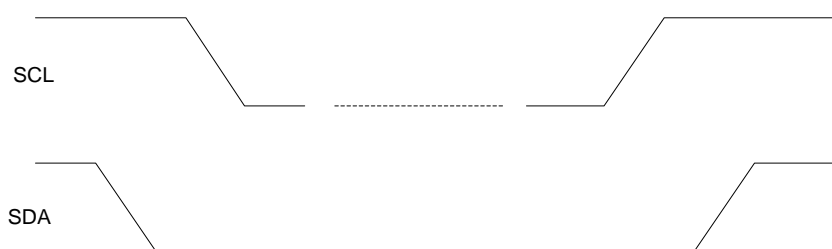
Figure 21 Timing of I2C START and STOP conditions
