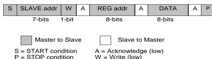
Figure 22: I2C byte write (SDA signal)
