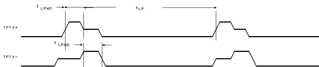
Transmitted Link Integrity Pulse Timing
