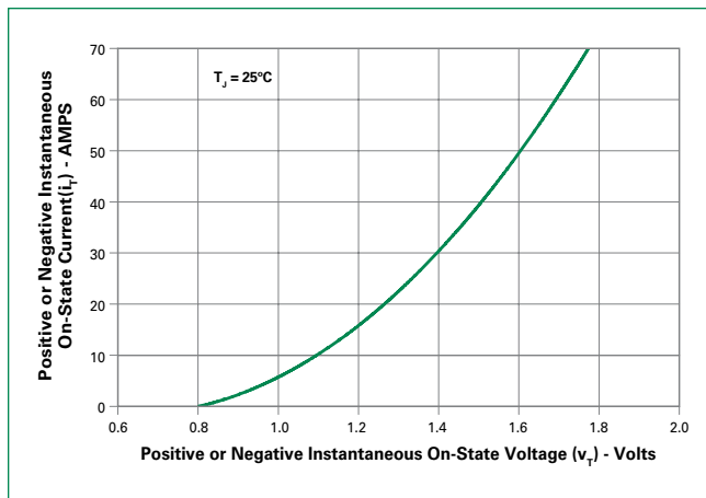
Figure 9: On-State Current vs. On-State Voltage (Typical)
