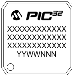
144-Lead TQFP (16x16x1 mm)
