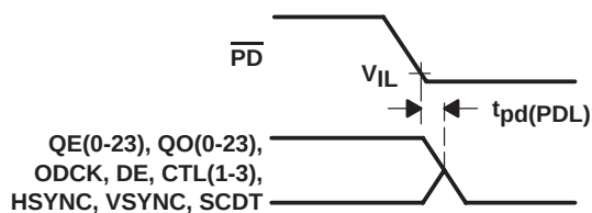
Figure 7. Delay From \overline{\text{PD}} Low to Hi-Z Outputs
