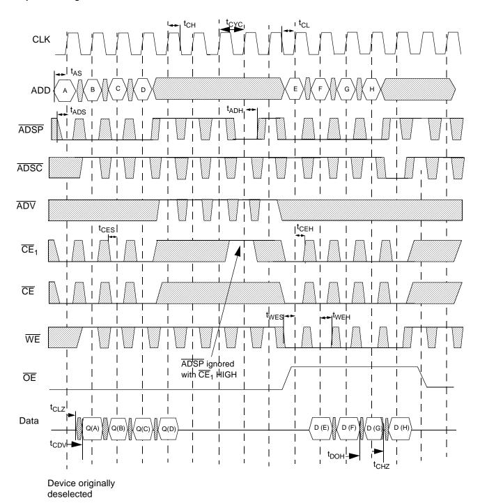
$\overline{\text{CE}}$  is the combination of  $\text{CE}_2$  and  $\overline{\text{CE}}_3$ . All chip selects need to be active in order to select the device. RAx stands for Read Address X, WAx stands for Write Address X, Dx stands for Data-in X, Qx stands for Data-out X.
