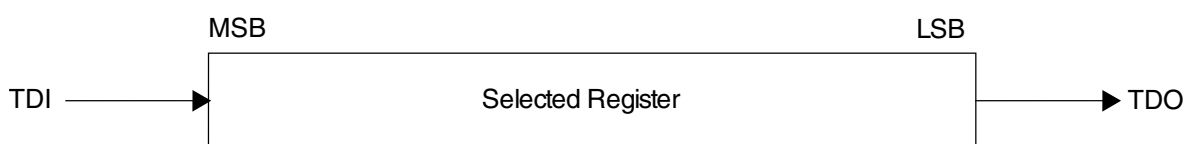
Figure 63-3. Shifting data through a register
