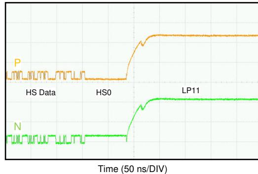
Figure 8-11. CSI-2 End of Transmission (EoT)
