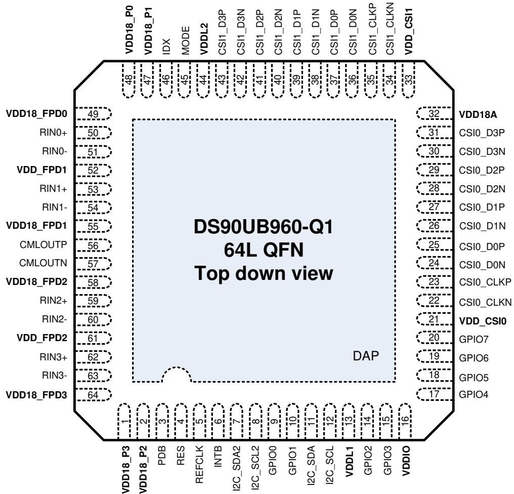
Figure 5-1. RTD Package 64-Pin VQFN (Top View)
