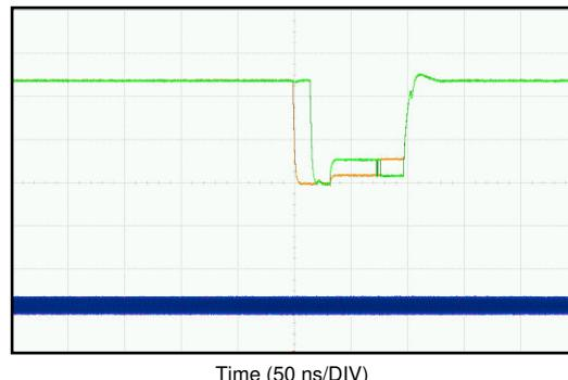
Figure 8-9. CSI-2 DATA and Continuous CLK Output
