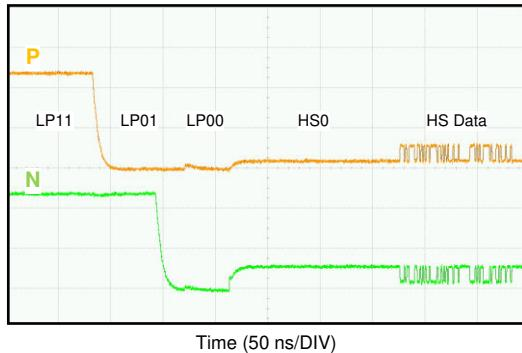
Figure 8-10. CSI-2 Start of Transmission (SoT)
