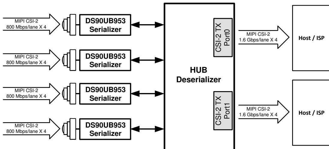
Figure 8-12. Four DS90UB953-Q1 Sensor Data Onto CSI-2 Over 2 Ports
