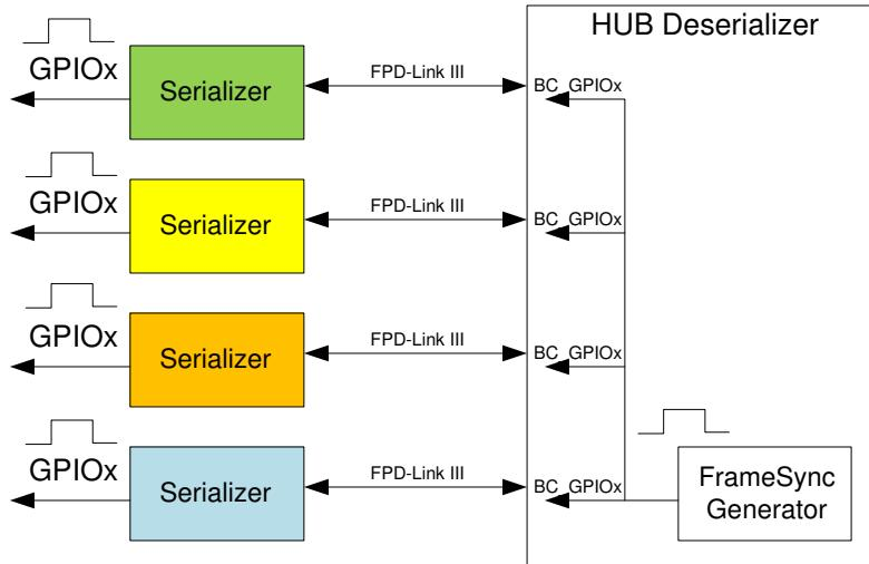
Figure 7-17. Internal FrameSync
