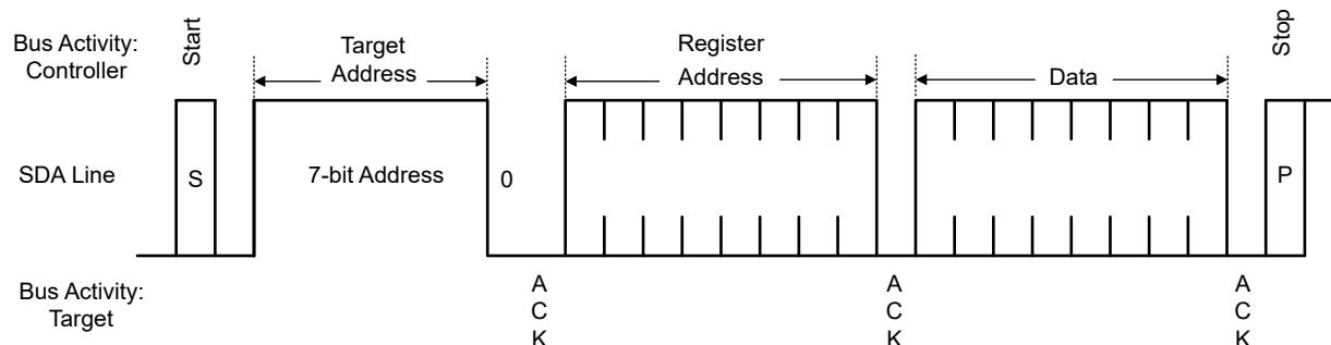
Figure 7-25. Serial Control Bus — WRITE
