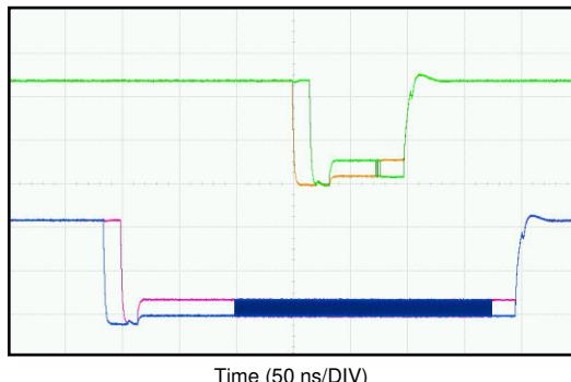
Figure 8-8. CSI-2 DATA and CLK Output
