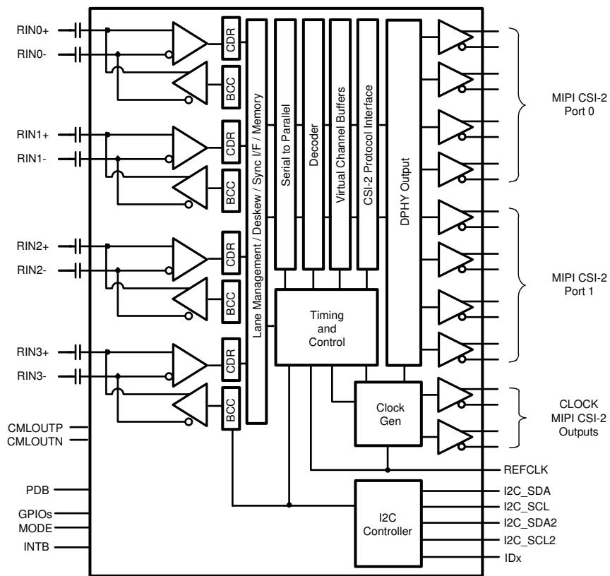
Figure 7-1. Functional Block Diagram
