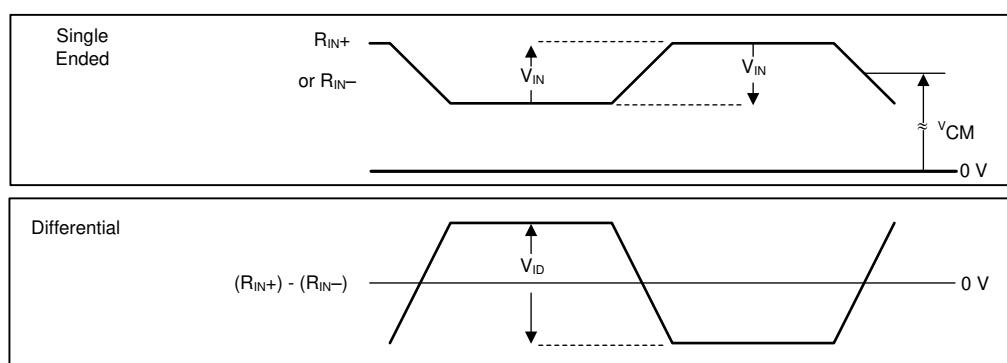
Figure 6-2. FPD-Link Receiver VID, VIN , VCM
