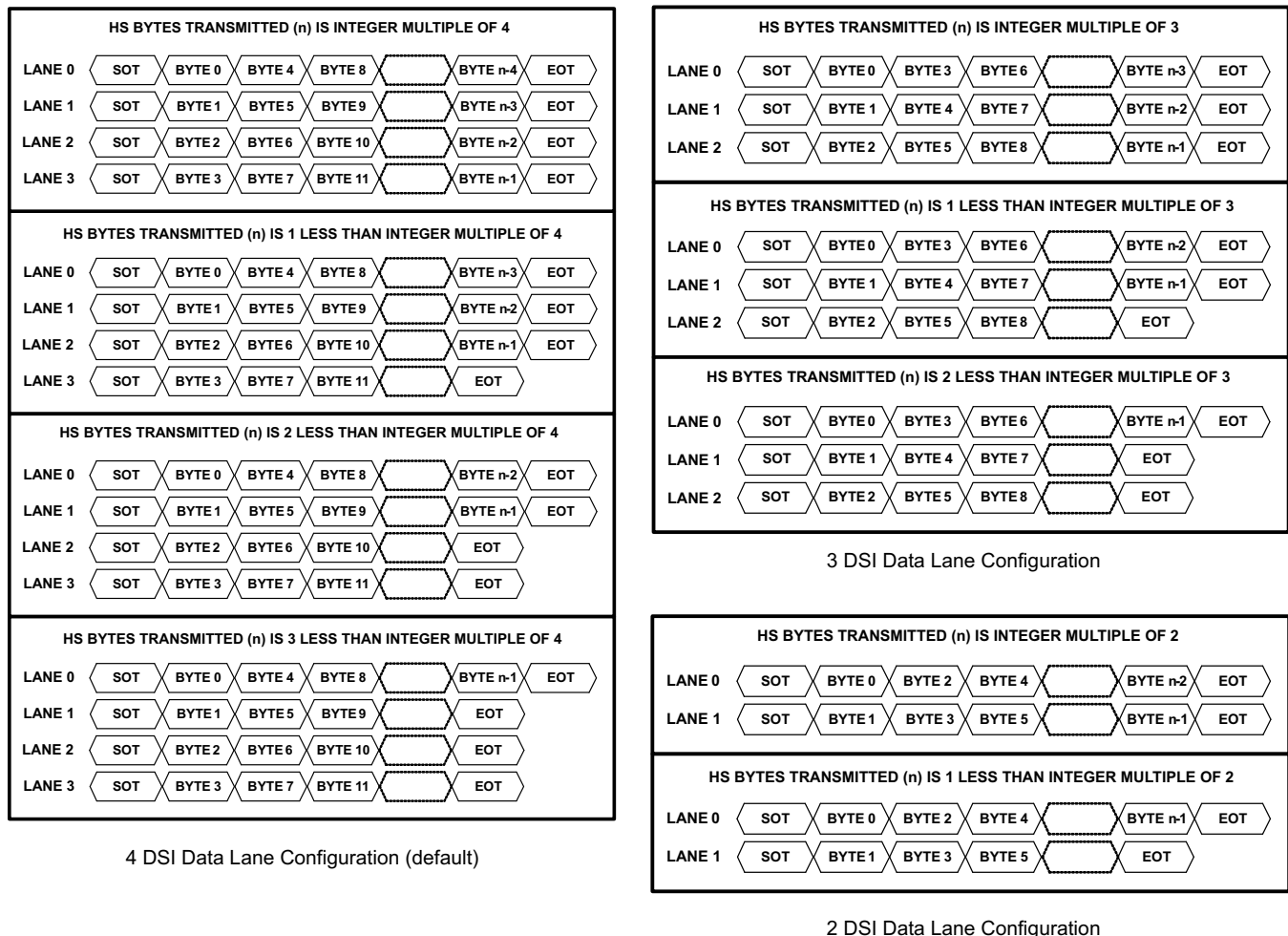
Figure 13. SN65DSI83-Q1 DSI Lane Merging Illustration
