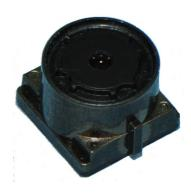
The Toshiba TCM9820MD is 8M pixels camera module with EDOF system. The optical format is 1/3 inch, of which small size is suitable for built-in camera module application. The full resolution is 3280 x 2464 pixels, and 1/2 binning mode for view finder is 1640 x 1232 pixels(Maximum size). The maximum frame rate with full resolution is 15fps, and 60fps for view finder is available.
