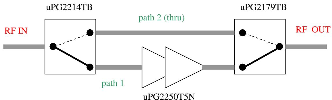
The two paths are selected by the logic levels at the two control pin-connectors, VA and VT, (refer to the schematic for the connector designation) according to the following truth table:
