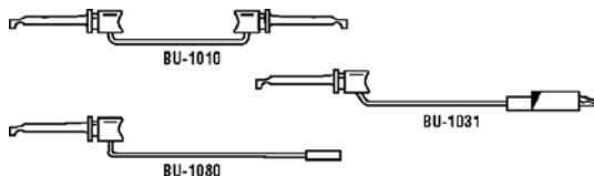
Type BU-1010 test leads make difficult IC connections fast and easy. Spring-loaded beryllium copper conductor attaches to component leads and terminals. Type BU-1031 test clip to insulated mini-alligator clip. Type BU-1080 test clip to 0.025" (0.635) square pin receptacle. Type BU-1111, mini-plunger clip.
