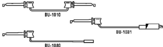
Type BU-1010 test leads make difficult IC connections fast and easy. Spring-loaded beryllium copper conductor attaches to component leads and terminals. Type BU-1031 test clip to insulated mini-alligator clip. Type BU-1080 test clip to 0.025" (0.635) square pin receptacle. Type BU-111, mini-plunger clip.
