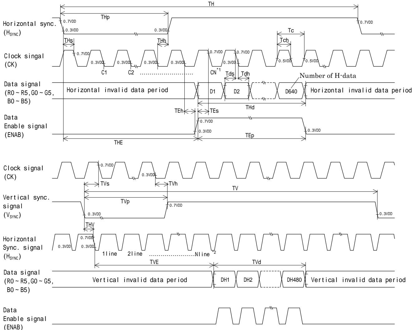
\*1 When ENAB is fixed at "Low", the horizontal display starts from the data of C144 (clock).
