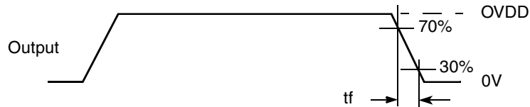
Figure 7. Definition of Timing for Standard and Fast-Mode
