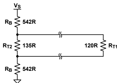
Figure 8. Single Fail-Safe Biasing for Short Data Links
