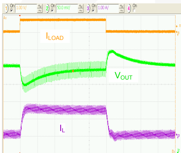
Figure 6. Load Transient Response, 1.2V OUT (100mA to 1500mA, 20µs/div)
