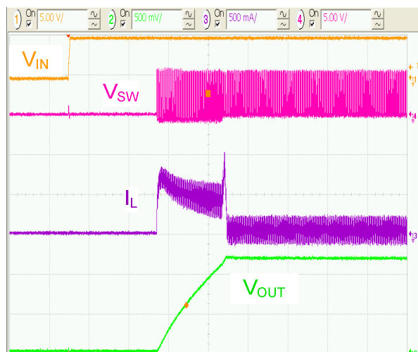
Figure 4. Startup with 100mA Resistive Load
