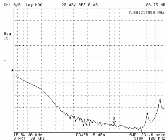
Figure 4 - Common Mode attenuation, 0.05-100 MHz. Source and load resistances are 50 \Omega . Two 0.47 \mu F Y-caps to common line. Vertical scale: 20 dB/div, with zero dB level marked by arrow.
