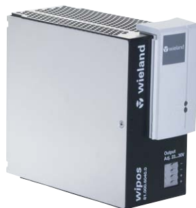
24 V / 10 A Primary switch-mode regulator €€; Approvals: , CSA and pending 70 x 153.5 x 164
