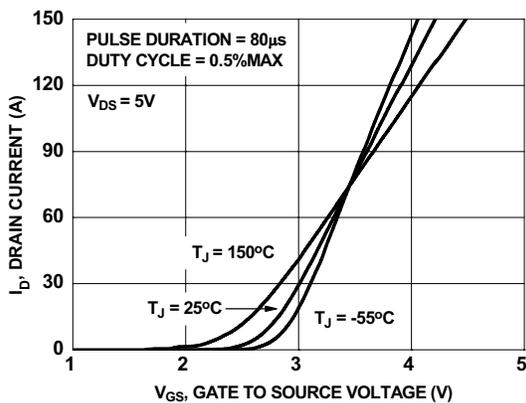
**Figure 5. Transfer Characteristics**
