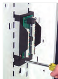
Step 2 - Secure with two screws
