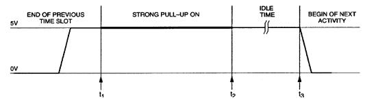
For infinite duration (Figure 9b) the strong pullup also begins immediately after the time slot is completed. To end the strong pullup, the DS2480B must receive a Termination command, code F1h, which occurs at t<sub>2</sub>. The termination command does not generate a response byte. The DS2480B will then immediately end the strong pullup and send out a pulse response byte. Everything else is the same as with predefined duration.
