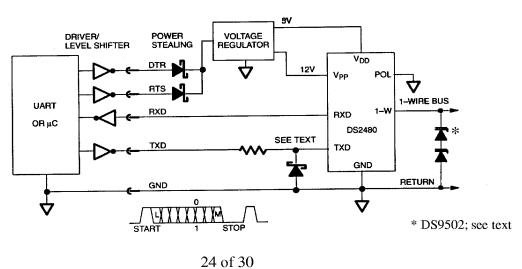
The signals DTR and RTS provide the power to operate the DS2480B. The resistor in the TXD line and the Schottky diode limit the negative voltage at the TXD pin of the DS2480B to 0.3V maximum. The resistor is typically 4.7 k $\Omega$ . If the inverting driver is current–limited to 1 mA the resistor is not required.
