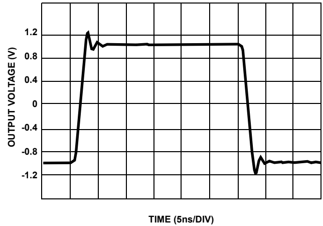
FIGURE 2. LARGE SIGNAL PULSE RESPONSE
